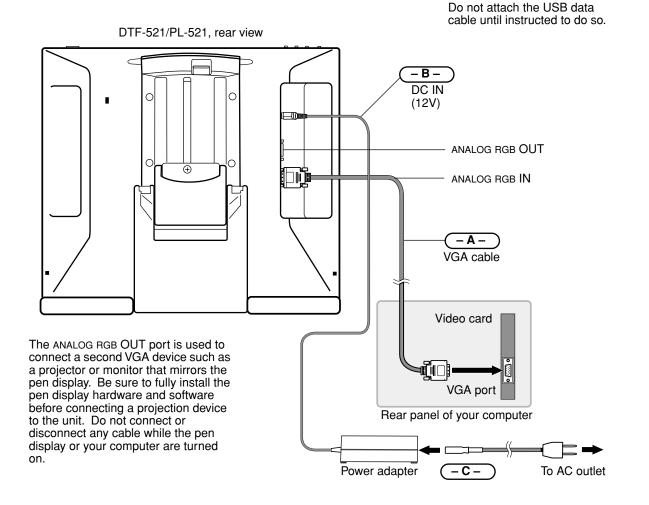
CAUTION Use only the power adapter that came with the DTF-521/PL-521; use of an improper power adapter may damage the unit.
